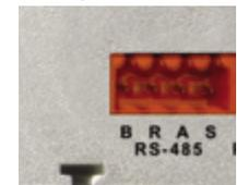
\*The reference pin is connected via 100 Ohm to the internal ground !
