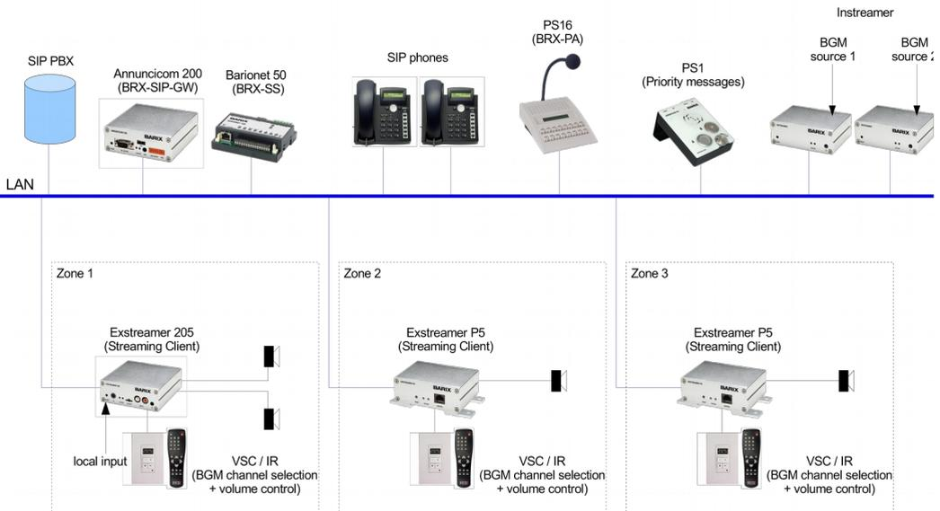
Being designed with a server/client architecture, the SIP ZONE PAGING application is configured to run on Barionet 50 (server), on PS16 (Paging Station) and on Annunicom 200 (SIP Gateway). As zone player can be used any Exstreamer/Annunicom device with BGM Client firmware or Streaming Client firmware.
