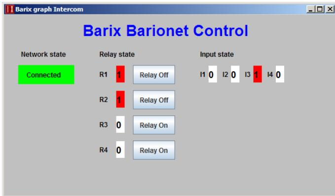
This example is extensively using the very powerful macro function and also dynamic labels. If you will use it with your Barionet, so change only the IP address in the ICgraph.cfg (PB) and define the UDP Control port 12301 on your Barionet setup.
