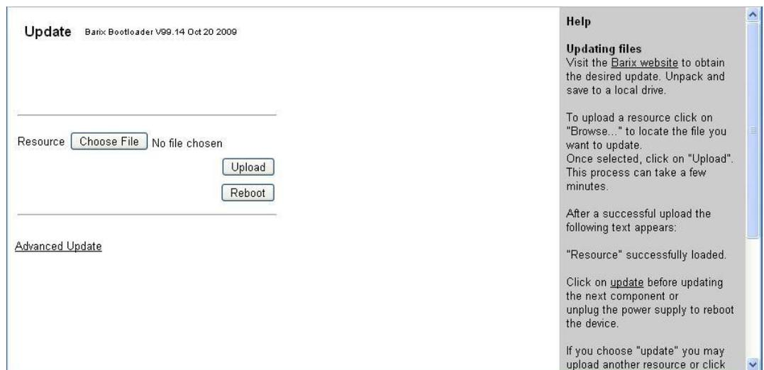
Figure 41. When the Barionet 50 restarts in Boot Loader mode, this Update screen appears.
