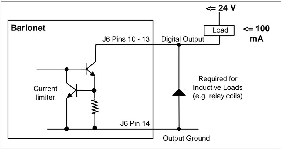
Figure 26. The open-collector digital outputs can sink up to 100 milliamps.
