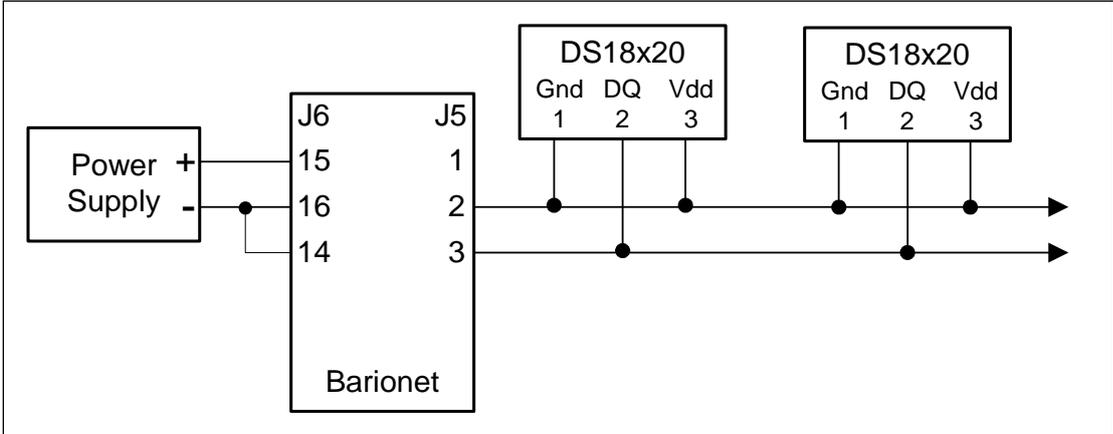
Figure 20. The first connection method for 1-Wire sensors.
