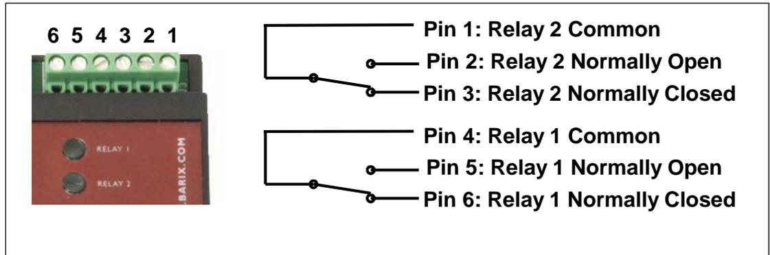
Figure 22. The Barionet Relay Outputs.
