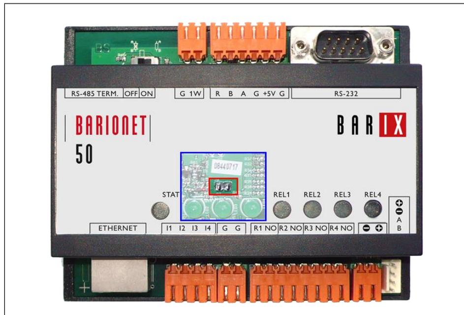
Figure 34. The Barionet 50 Reset jumper is under the lid near the RS-232 LED
