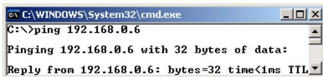
Figure 4. If the address assignment was successful, the response should look like this.
