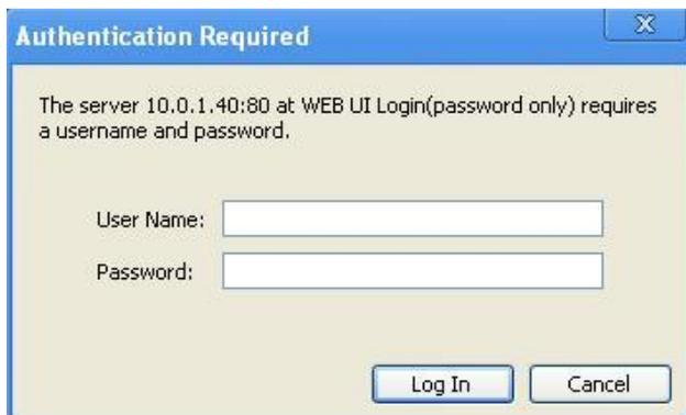
Figure 18. The authentication dialog appears when a user tries to access configuration pages when a password has been set.
