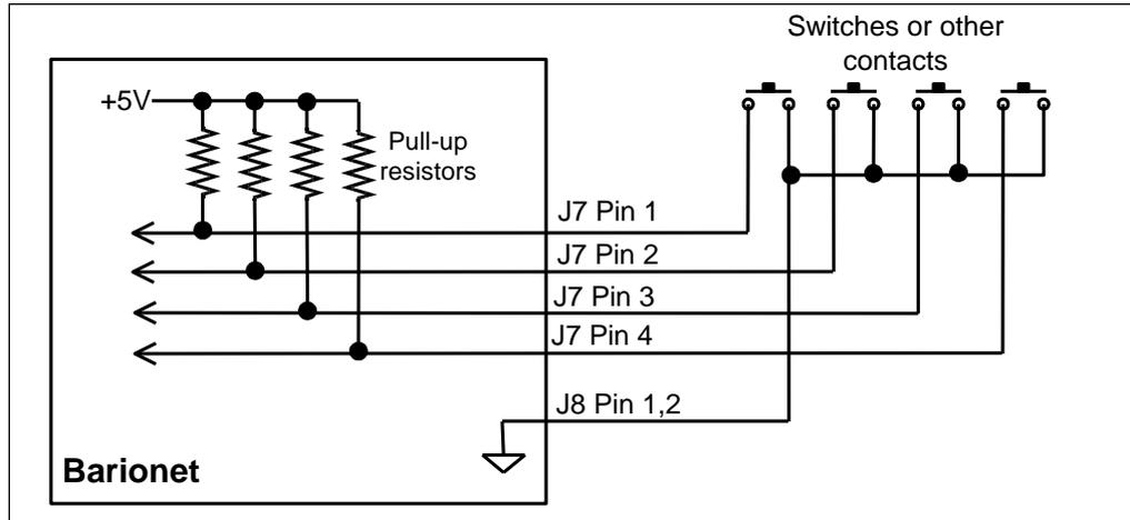
Figure 30. The Barionet 50's four digital inputs are designed to be used with switches or other contacts that connect to ground.
