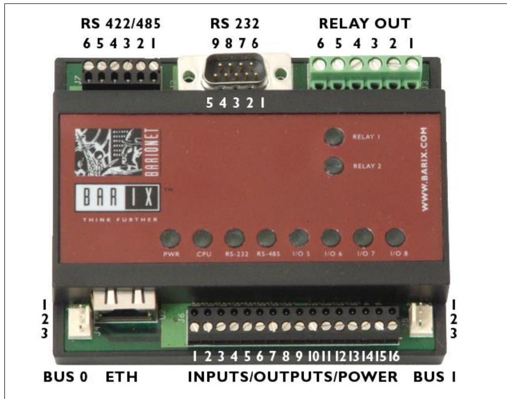
Figure 19. The Barionet 100 connectors and indicator lights.
