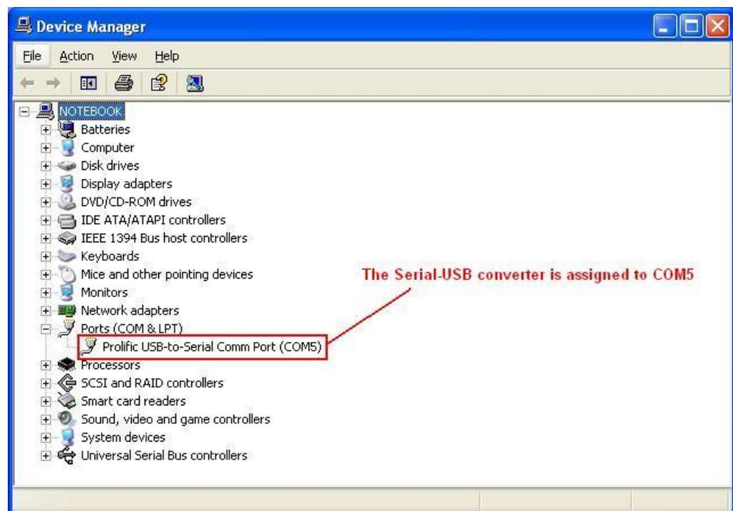
Figure 37. The Device Manager showing a USB-Serial adapter on COM5
